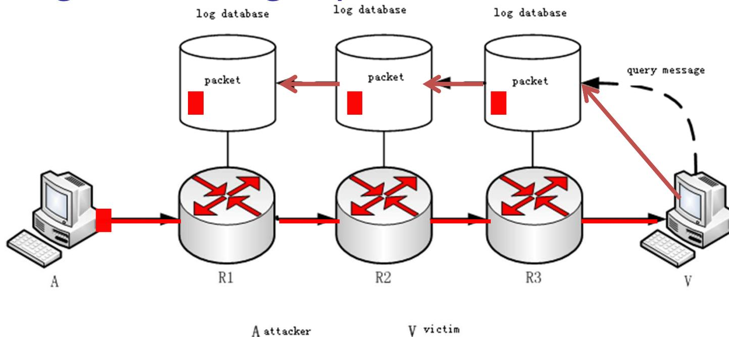
**Packets are logged by the routers on the path toward the destination. The network path is then derived based on the logged information. This approach is also known as SPIE.**
